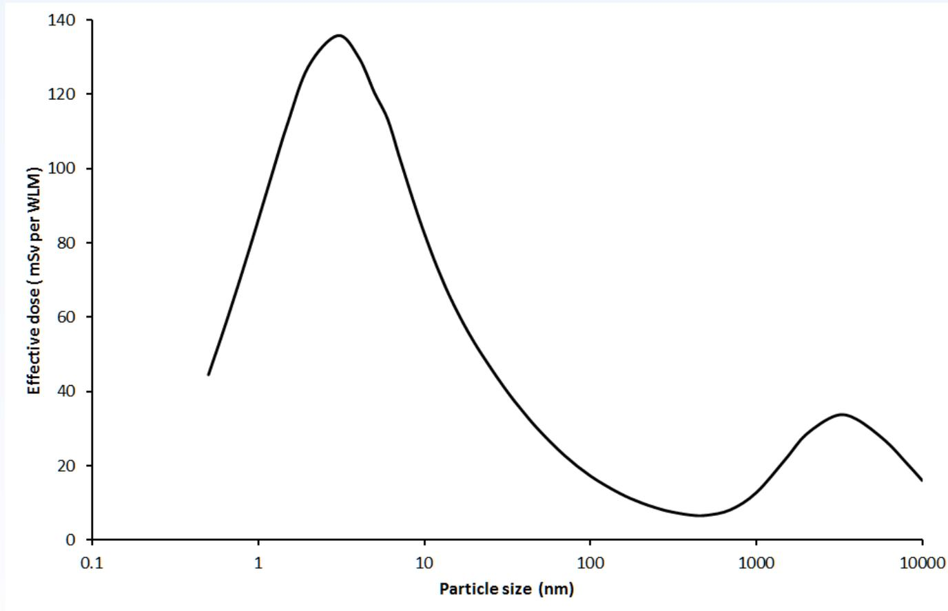
**Figure A.5.** Effective dose per WLM as a function of particle size of a monodisperse aerosol for a Reference Worker with an average breathing rate of  $1.2 \text{ m}^3 \text{ h}^{-1}$  following exposure to radon ( $^{222}\text{Rn}$ ) progeny. Unit density and unit shape factor were assumed and hygroscopic growth was not taken into account.
